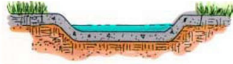
Figure 10.4.1 Traditional Infiltration Basin (Improving Stormwater Basin Design, 2008)
