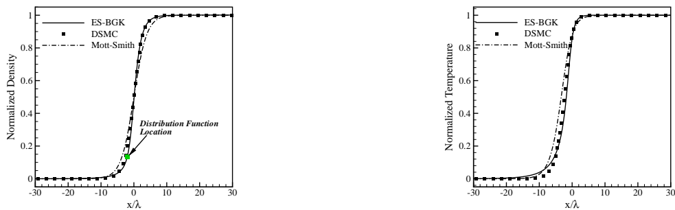
FIGURE 4. Comparison of normalized density and temperature profiles obtained using various methods for M = 2.5
