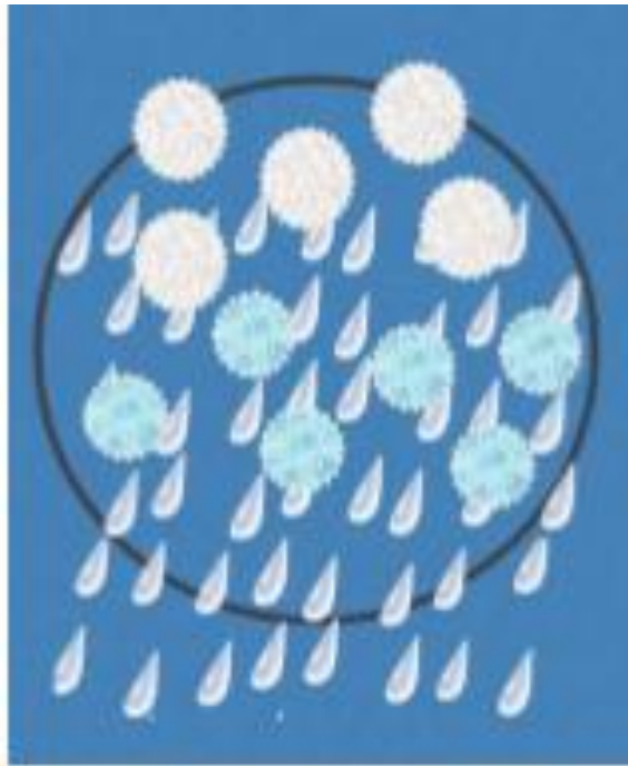
Fig. 3.1: A non-uniform mixture can produce a gradient of precipitation types within a radar beam (black circle). Mostly hail is sampled at the top of the beam, the middle is sampling rain and wet hail, and the bottom of the beam is sampling rain only (taken from WDTD 2013).
