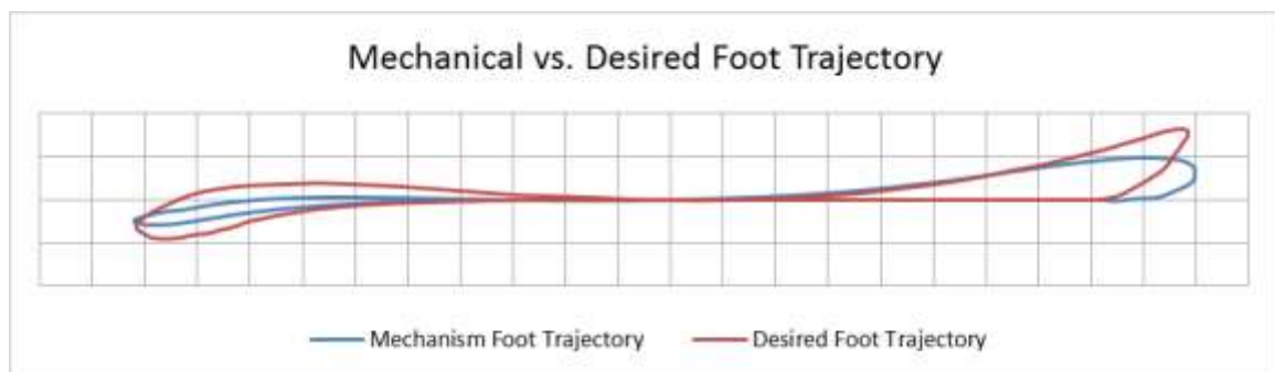
Figure 79. Mechanical vs. Desired Gait Trajectories
