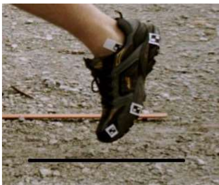
Figure 20. Height of Toe at First Peak (Initial Swing)
