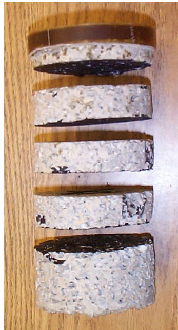
Epoxy Added and Specimen Sectioned Using Diamond Bladed Saw
