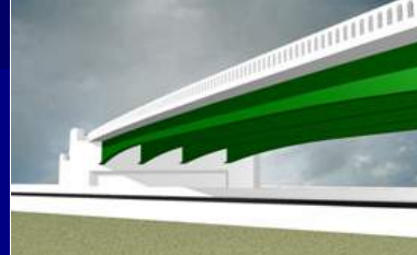
Variable Depth Steel Plate Girders
