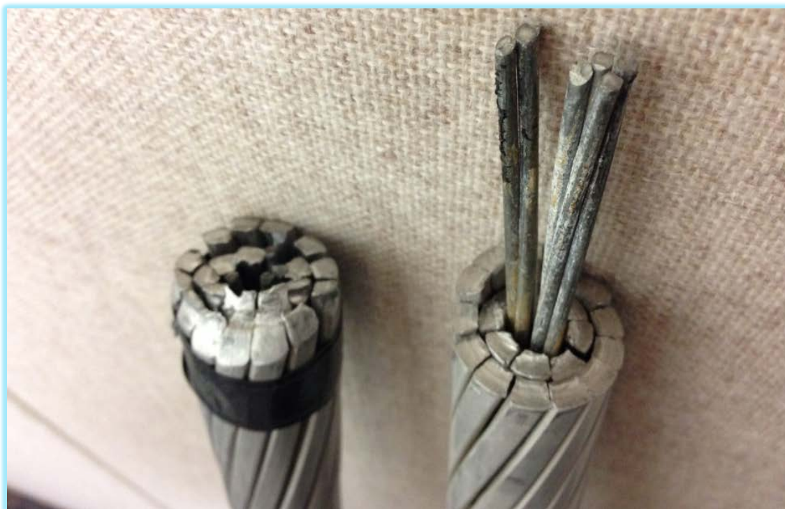
Figure 5 –Example of 954 Type 7 self-damping ACSR installed on over 1400 miles on the NPPD transmission system, center steel strands extended
