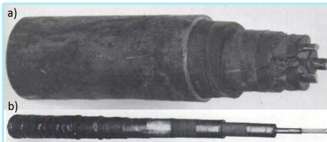
Figure 2 - a) Three-core 20kV paper insulated clover leaf cable b) Cables de Lyon continuous current cable, 1905
