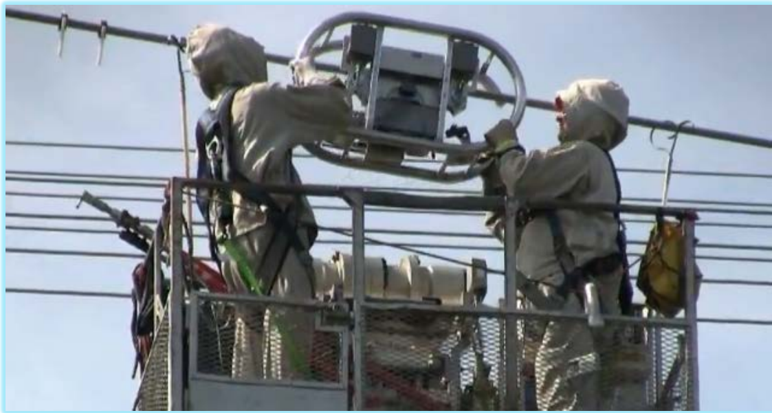
Figure 19 – NDE device used for condition assessment of ACSR conductor
