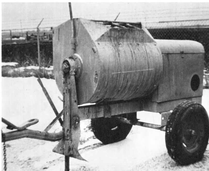
Figure 21. Highway maintenance crews used this typical mortar or plaster mixer for mixing concrete and/or mixing asphalt emulsion and/or slurry mixtures. This was one of the mixers we utilized later on in other crack filling activities. The only modification necessary was the addition of a tapered, threaded tap made in the bottom of the drum so that an elbow, valve, and reservoir could be placed underneath this outlet to control the discharge of the slurry which then was picked up by the pneumatic pump and pumped into the pavement cracks. The pumpable slurry crack sealing mix was designed in our bituminous laboratory and the best formulation for this pumping operation involved a 50% limestone aggregate and a 50% CSS-1 emulsion by weight.
