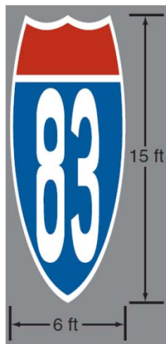
A - Interstate Shield on dark or light pavement
