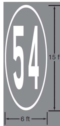
D - State Route Shield on dark pavement
