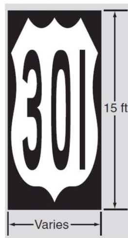
C - U.S. Route Shield on light pavement
