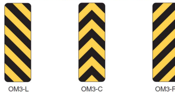
Type 3 Object Markers (obstructions adjacent to or within the roadway)
