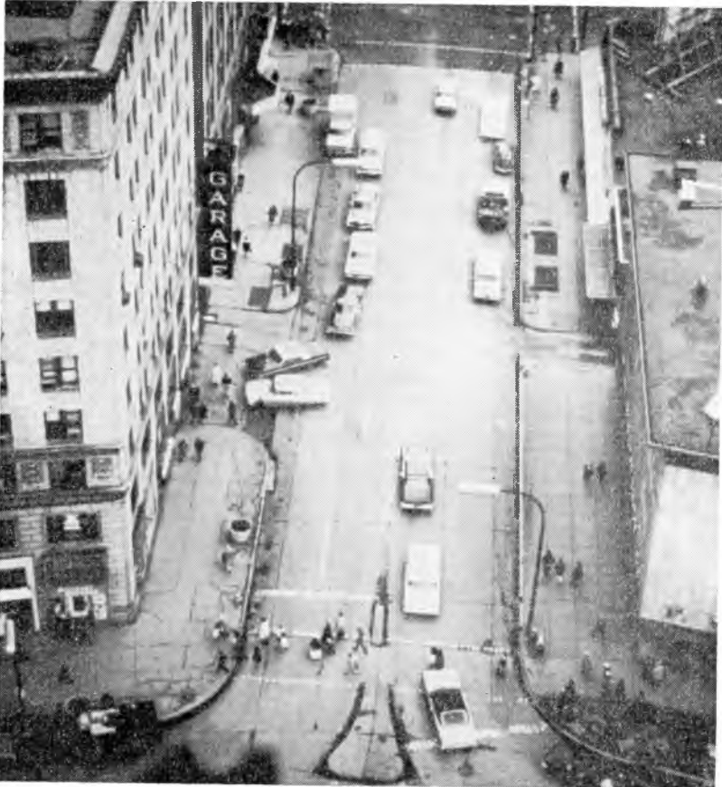
Fig. 5. Parked truck keeps the curb lane from being used as storage lane for right turns into facility.
