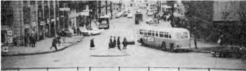
Fig. 1. Drive located too near intersection where left turns are being made. Turning vehicles block bus across crosswalk.
