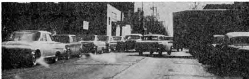
Fig. 9. Parking permitted on both sides of a narrow street, resulting in street being blocked during maneuvering of vehicles.
