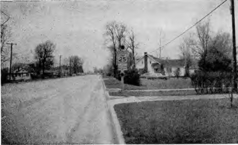
Fig. 5. Traffic control device used—special speed limit sign with vertical alternate flashing signals.
