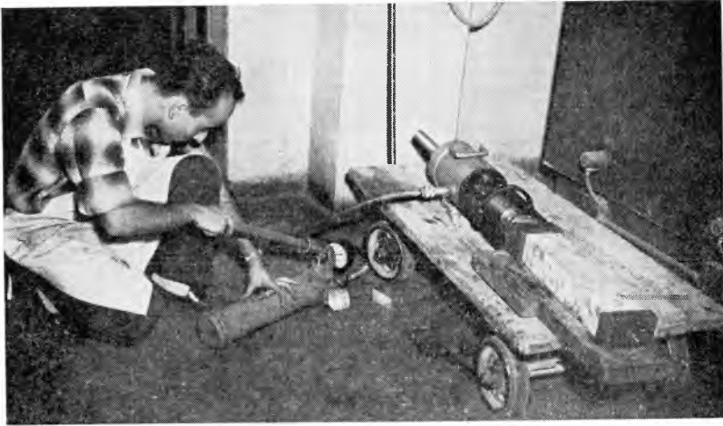
Fig. 1. Sixty-ton hydraulic jacking unit and specimen in position for post-tensioning.
