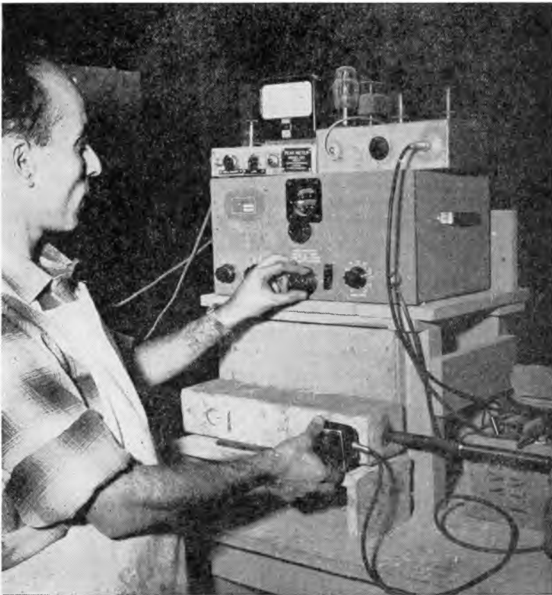
Fig. 3. The natural frequency apparatus and specimen in position for testing.
