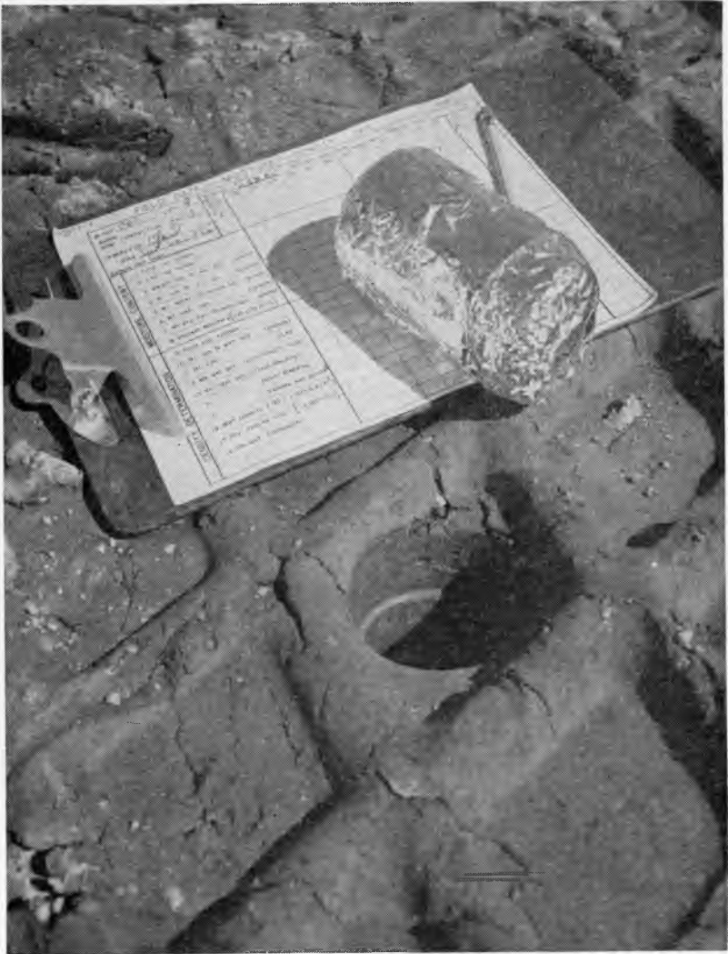
Fig. 6. Many samples were taken in each compacted lift in the top three feet of the AASHO Road Test embankments to insure close control of the density and moisture content. Here a field density sample has been taken and wrapped in foil for its trip to the Materials Laboratory.
