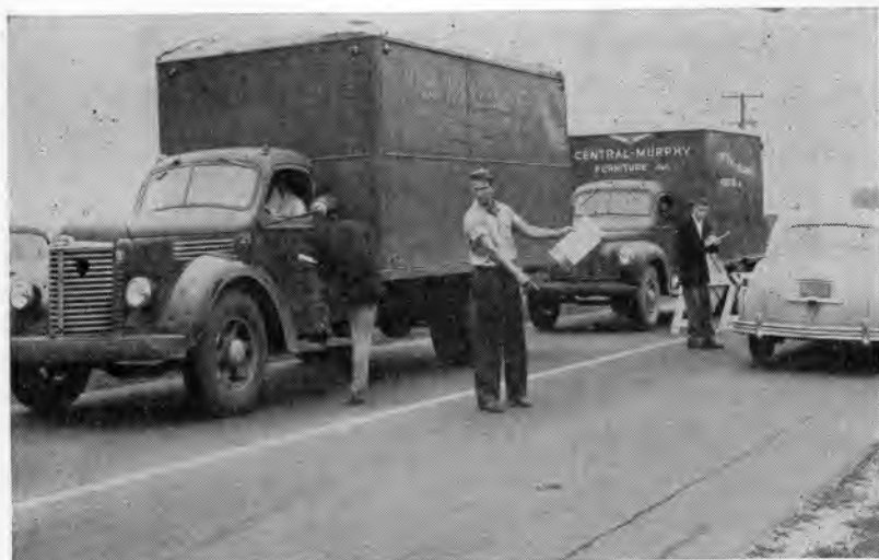
Fig. 23. Data for research and planning are being obtained through origin and destination surveys as illustrated in this view. (23448)
