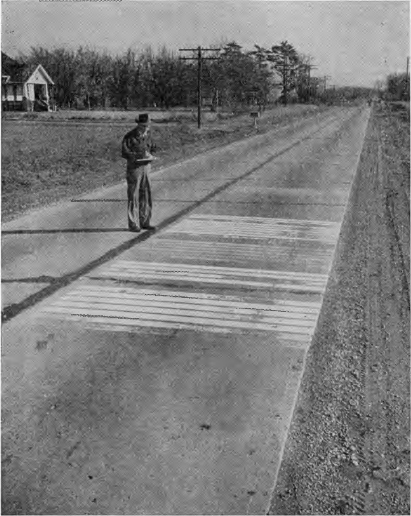
Fig. 16. Field testing of traffic paints for the Highway Department is illustrated in this view. Note the wide range in quality of the various paints being tested. (3265)
