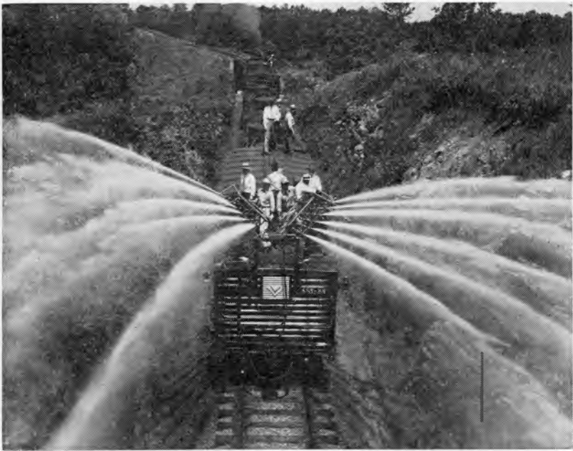
Fig. 3. Chemical weed control will save America's railroads millions of dollars in maintenance costs.
