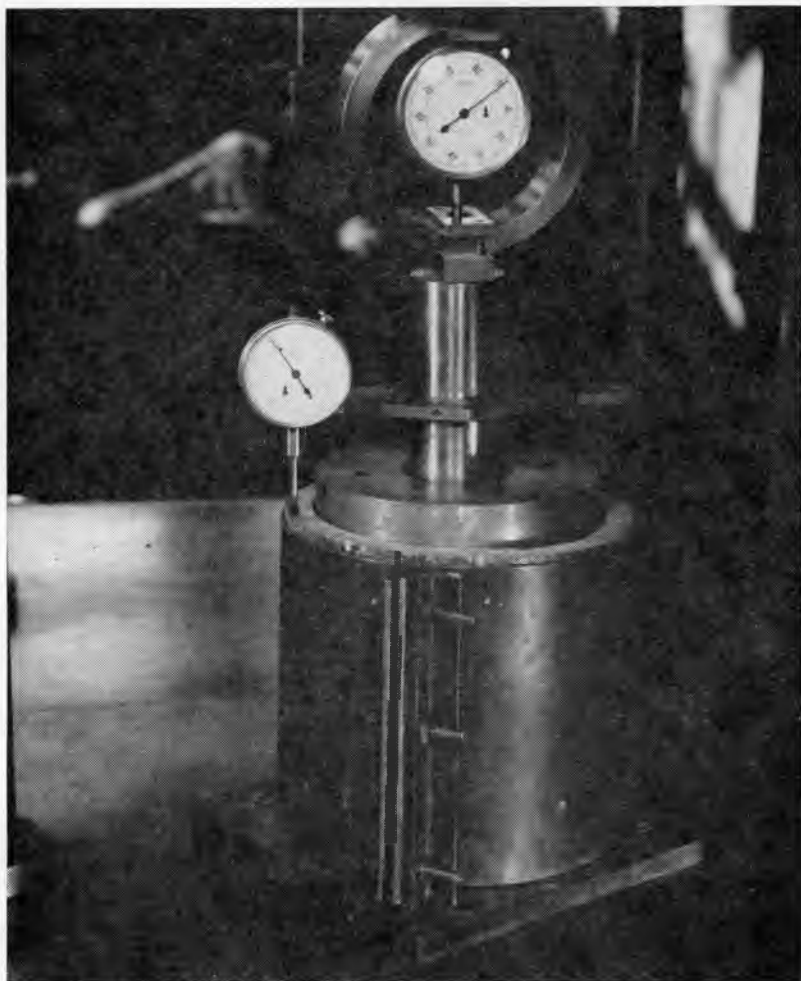
Fig. 1. Equipment set-up for laboratory C. B. R. test. The clay cylinders were reinforced with a metal casing.
