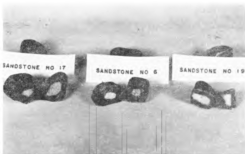
FIGURE 8. Sandstone broken open at the completion of the asphalt absorption test, showing the extent of asphalt absorption.
