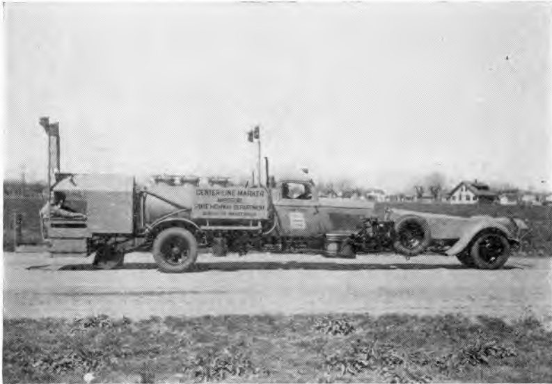
Pavement marker built by the Equipment Bureau of the Missouri State Highway Department.
