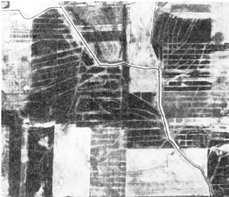
Fig. 7. An aerial photograph showing the location of subsurface tile drains through the medium of color tone.
