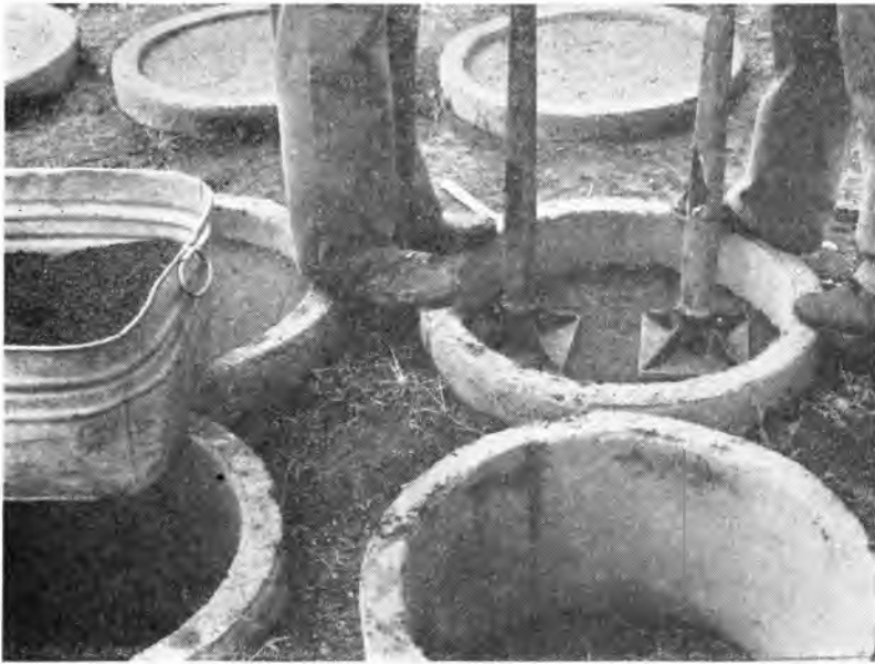
Fig. 4. Close-up of experiment shown in Fig. 3, illustrating the tile and method of installing fixtures in the tile.
