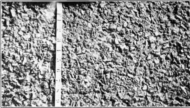
Fig. 6. Surface texture of penetration macadam, A-5 type, as shown in Fig. 5.
