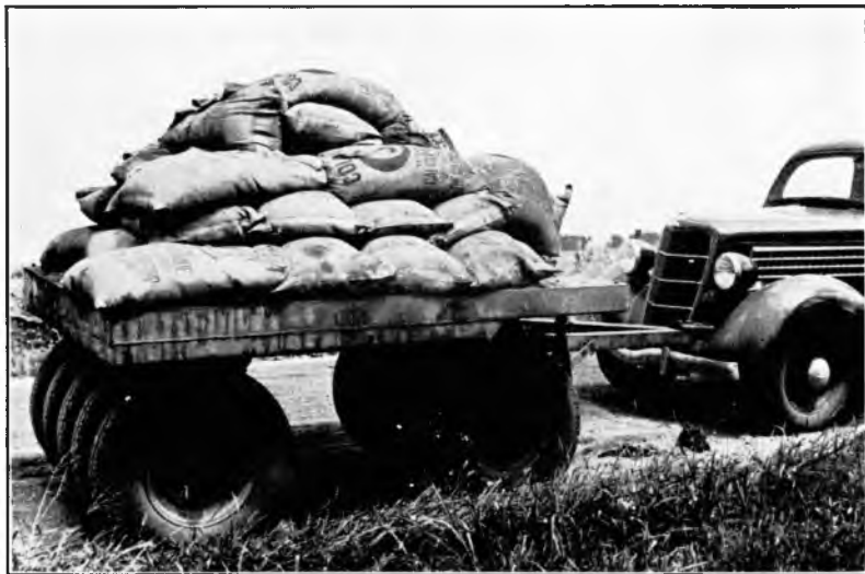
Fig. 6. Multiple pneumatic-tired roller used in Illinois. This type of roller provides both a kneading and a compacting action.
