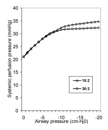
Figure 1. Systemic perfusion pressure during ITPR-CPR for various negative airway pressures with 100 chest compressions per minute and two regimes of positive pressure ventilations (15:2 and 30:2). Systemic perfusion pressures are average values for first 60 sec of CPR after cardiac arrest. Thoracic pump factor = 0.75. The abscissa indicates negative airway pressure.
