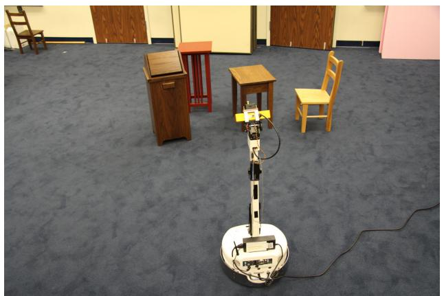
A robot (Čapek), equipped with a stereoscopic camera, is tasked to recover the 3D scene in front of it, and then plan and execute navigation tasks within it.
