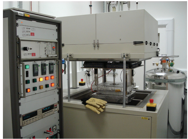
Figure 2. Schematic diagram of the low temperature GHP used by National Physical Laboratory (NPL).
