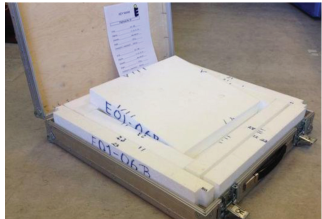
Figure 3. Example of test specimens cut down to 400 × 400 mm.
