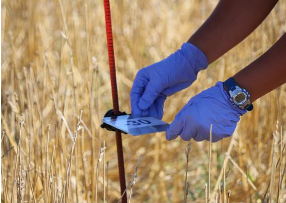
Fig. 6.1. A drift collection station used for the trial in 2013. A mylar cards is held in place by a paperclip on a metal platform, which is held up by a metal pole and clip. The mylar cards were placed at a level just above the wheat stubble.
