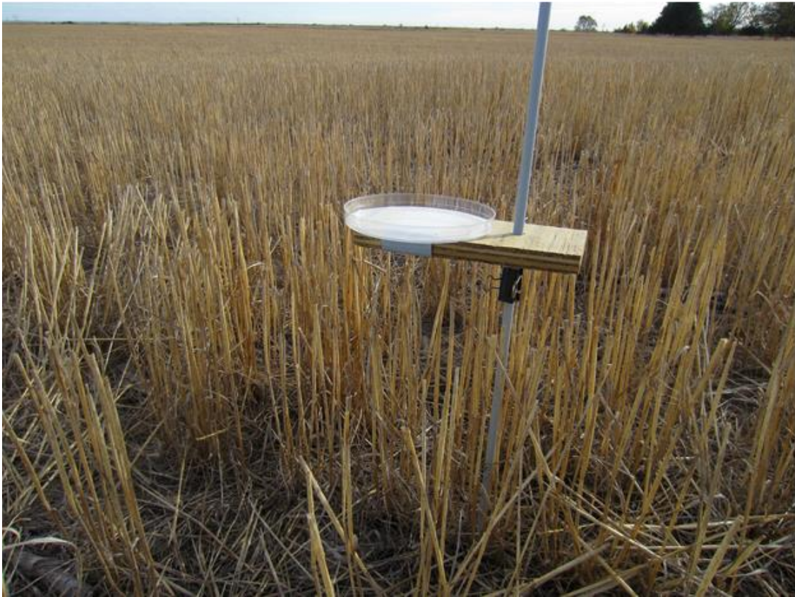
Fig. 6.2. A drift collection station used for the trial in 2012. A petri dish is held in place by tape to a wooden platform, which is held up by a fiberglass pole and clip. The petri dishes were placed at a level just above the wheat stubble.
