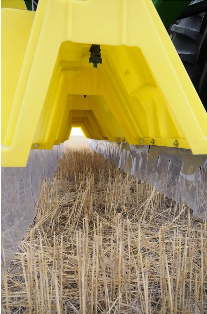
Fig. 6.4. The hood design used in the 2012 trial. The hood consisted of molded plastic extending approximately 30.5 cm below the nozzle orifices, and the plastic curtain extended approximately 10.2 cm below the hood.
