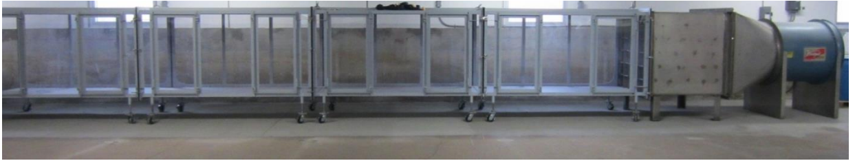
Figure 5.1. The low-speed wind tunnel used at the Pesticide Application Technology Laboratory in North Platte, NE. The axial flow fan at right is the source of the wind, which travels through the expansion chamber, air straightener, and 1.2 x 2.4 m sections. The scrubber system (not pictured) sits at the terminal end of the tunnel, 14.6 m from the air straightener.
