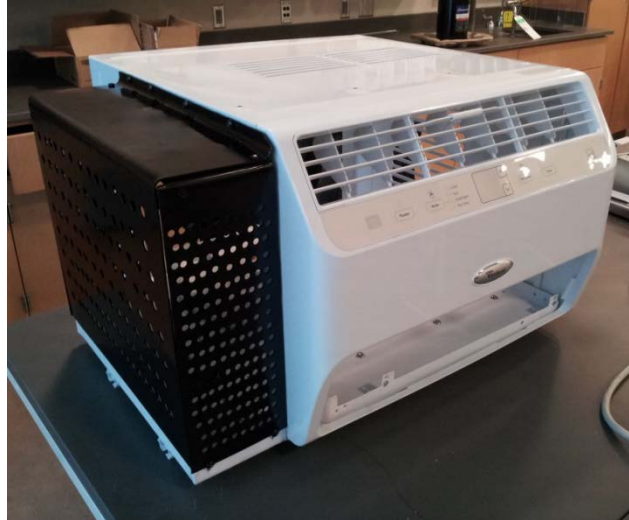
Figure 3: RAC housing expansion to accommodate compressor for R-1234yf system
