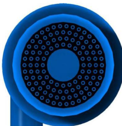
Figure 2: Cross section of the 116 tubes mini-channel heat exchanger. The internal diameter is 0.5 mm; the shell side hydraulic diameter is 1.8 mm.
