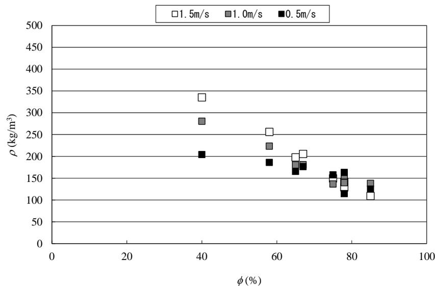
**Figure 4:** The obtained frost layer as a function of the relative humidity with different inlet air velocity.
