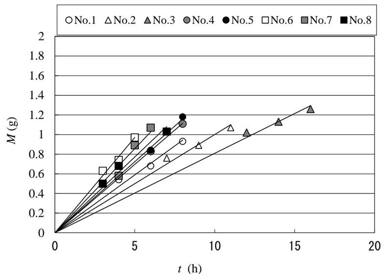
**Figure 2:** The measured frost mass as a function of time at  $u=1.5$ .
