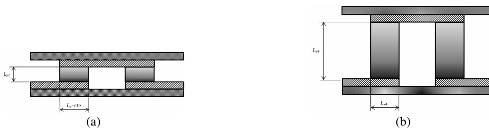
Figure 9: Samples of geometries analyzed in case of constrained base area: (a) aspect ratio 1/2, (b) aspect ratio 2
