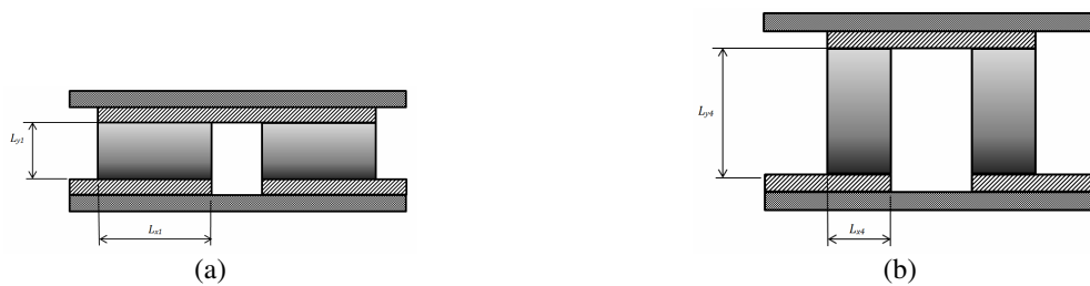
Figure 10: Samples of geometries analyzed in case of constrained volume: (a) aspect ratio \frac{1}{2} , (b) aspect ratio 2
