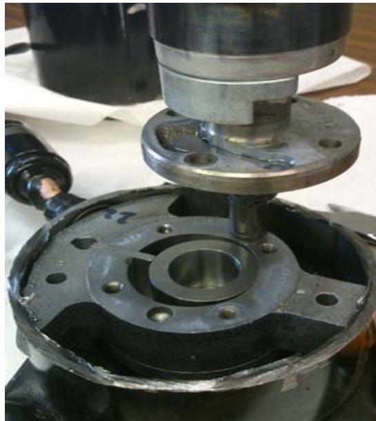
Figure 3. Dissected rotary compressor after experiments.
