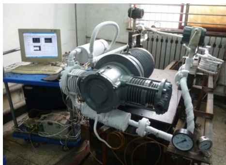
Figure7: Running experimental compressor and test rig
