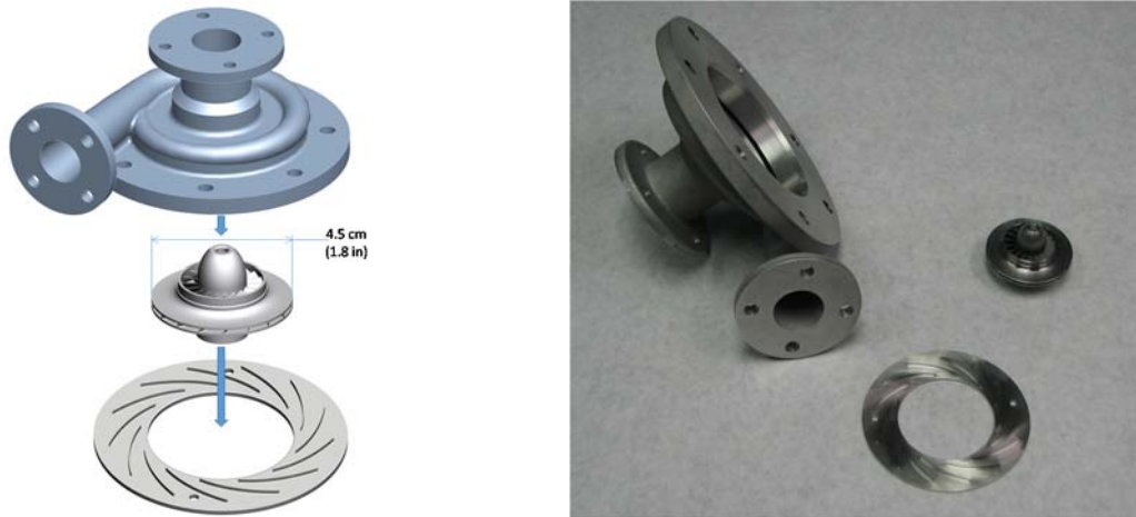
Figure 2: Final Design and Prototype Aero Parts - Volute Housing (Top) Impeller (Middle) and Diffuser (Bottom)
