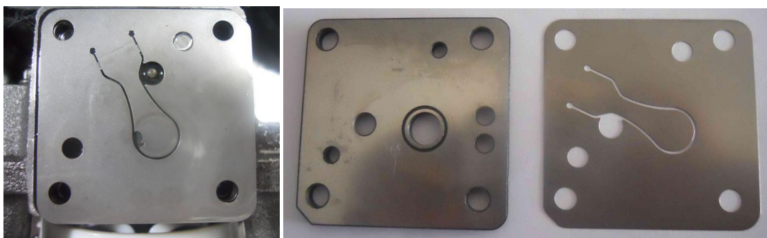
Figure 11: a) A failed valve in modified AISI 420. b) A well-functioning valve in Sandvik Hiflex™.
