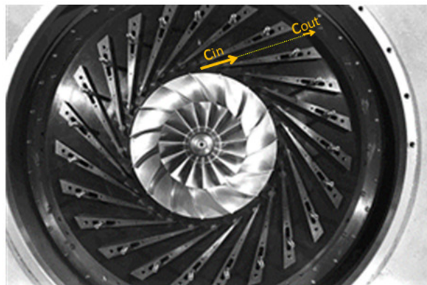
Figure 3: Vaned diffuser mean streamline showing a larger velocity reduction and a shorter passage length
