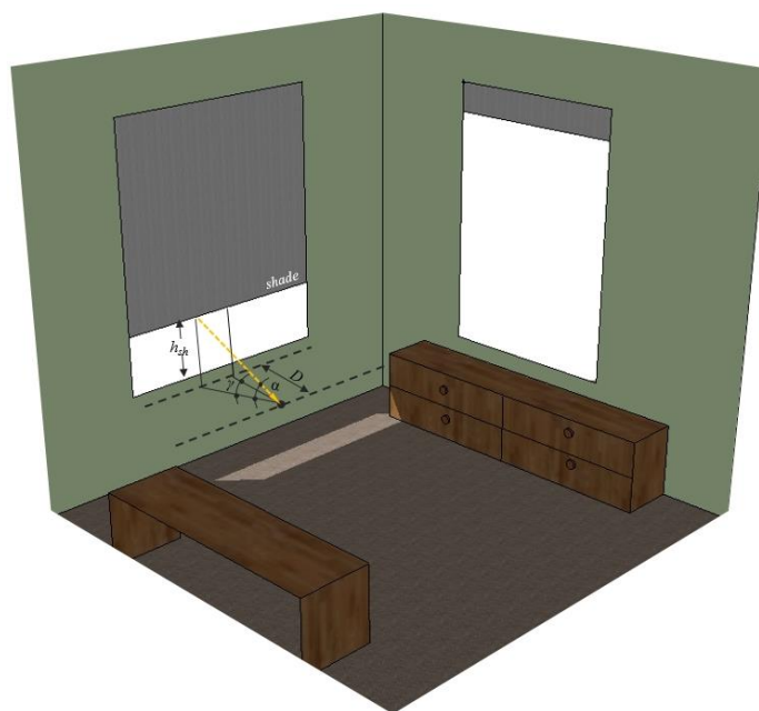
Figure 1: Graph showing shading position to prevent direct sunlight falling on the work plane area close to the occupant at all times
