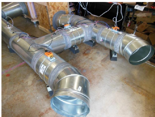
(a) air-side economizer configuration
