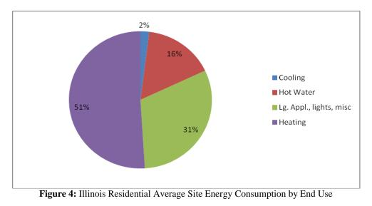
The most noticeable difference between the two is the dissimilarity between the percentage of the consumption due to the heating in the two cases, 72% for the test house and 51% for the average residential home in Illinois. As highlighted before the test house is essentially uninsulated. Thanks to the analysis, it is possible to understand early on that the majority of the energy savings will come from the retrofit of the envelope.
