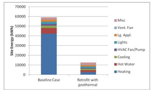
Figure 7: Predicted Annual Site Energy Use (kWh) of Optimum Retrofit with Geothermal Heat Pump
