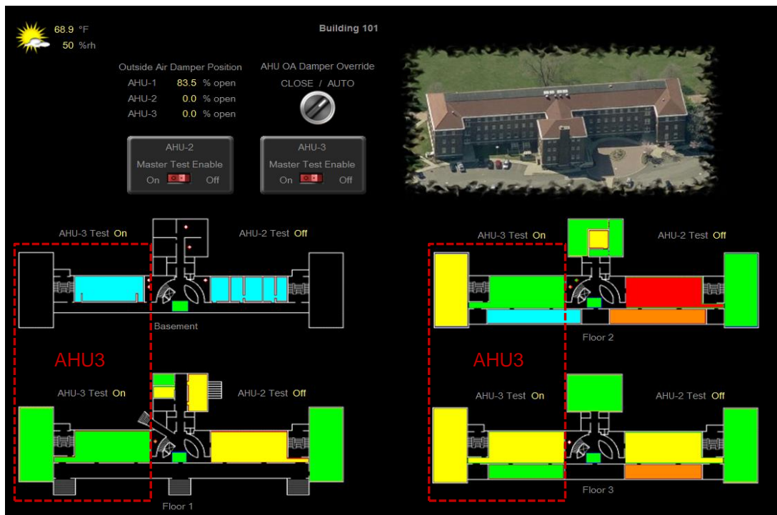
Figure 1: WebCTRL view of Building 101 zones
