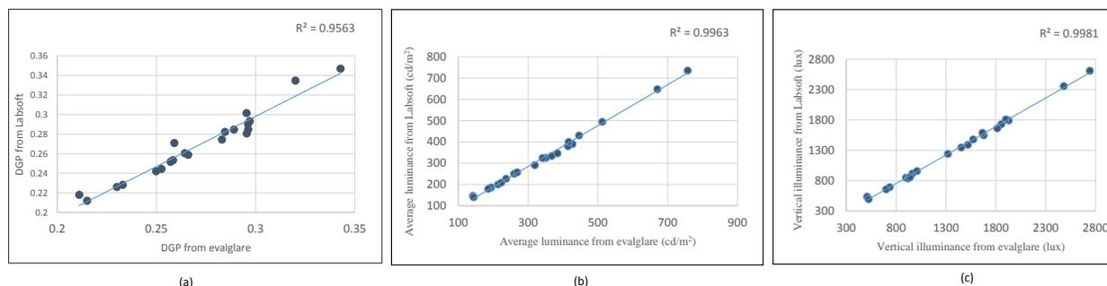
**Figure 2:** Validation for Labsoft's (a) DGP, (b) average luminance and (c) vertical illuminance using Evalglare as a baseline.
