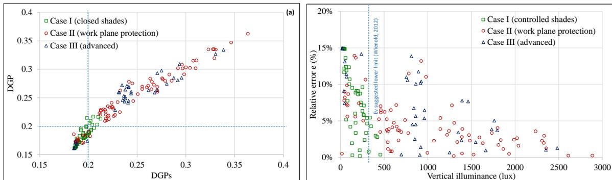
**Figure 9:** (a) Comparison between DGP and DGPs for all cases considered. – (b) DGPs relative error as a function of vertical illuminance for all studied cases
