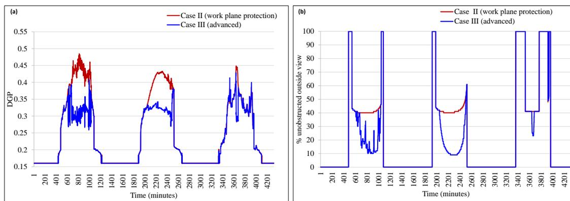
**Figure 11:** (a) DGP variation during comparative shading control experiments – (b) Percent of unshaded window area (unobstructed outside view during the comparative shading control experiments).
