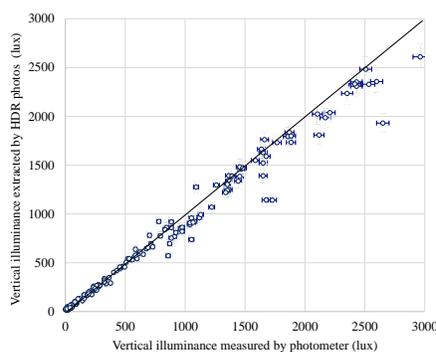
**Figure 3:** Validation of Labsoft's vertical illuminance using a camera-mounted illuminance meter for the case of controlled shades. ( $R^2=0.9817$ )
