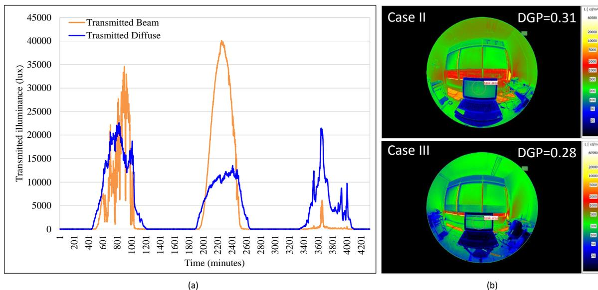
**Figure 10:** (a) Transmitted direct and diffuse illuminance during the comparative experiments. (b) Sample simultaneous luminance mapping for the two shading control strategies (first day, 4:30pm)
