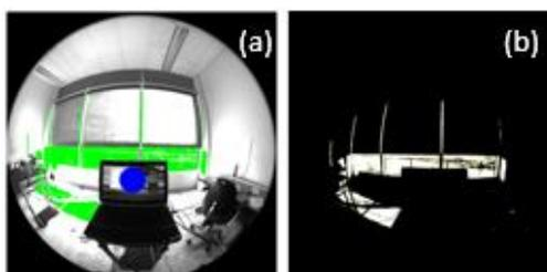
**Figure 4:** Glare sources identification through (a) Evalglare and (b) Labsoft (sunny conditions, employed shades (DGP=0.23)).
