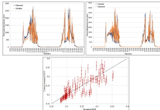
**Figure 5:** Validation of the model for (a) vertical illuminance; (b) work plane illuminance and (c) DGP (MSE=0.03)
