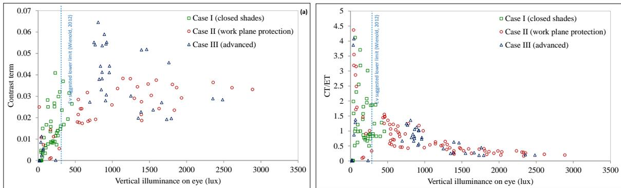
**Figure 8:** DGP contrast term as a function of vertical illuminance: (a) absolute value – (b) relative value (divided by the vertical illuminance term)
