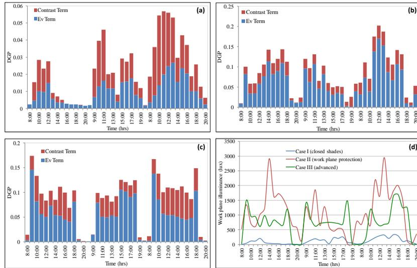
**Figure 7:** Contribution of vertical illuminance and contrast term for the three control cases: (a) Case I; (b) Case II; (c) Case III and (d) Work plane illuminance using the three shading control strategies for representative days used to study the effect of vertical illuminance and contrast terms.
