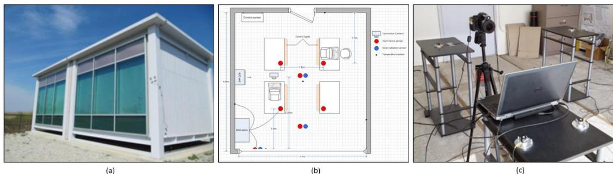
**Figure 1:** (a) Exterior view of the twin labs – (b) Sensors placement in the experimental room – (c) Interior view
