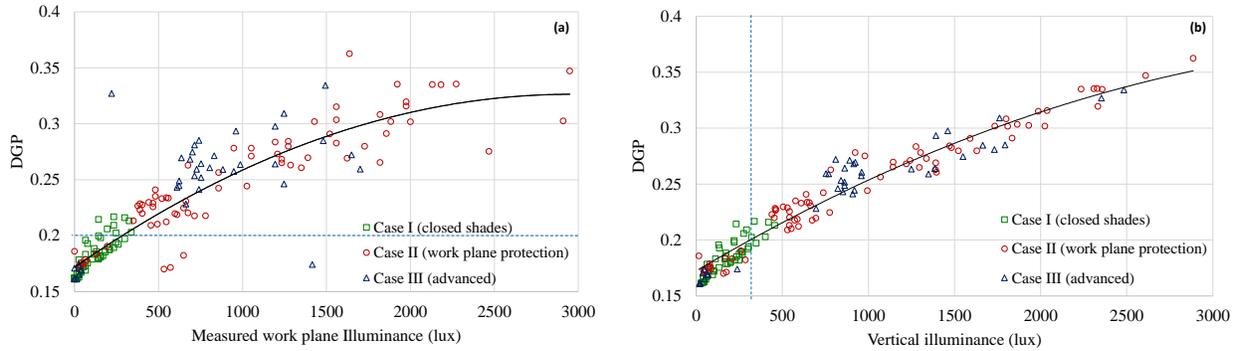
**Figure 6:** Correlation between measured DGP and (a) work plane illuminance and (b) vertical (eye) illuminance
