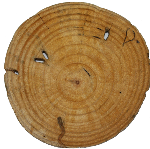
Fig. 3. An example of damage caused by beetles in a partially protected bolt.
