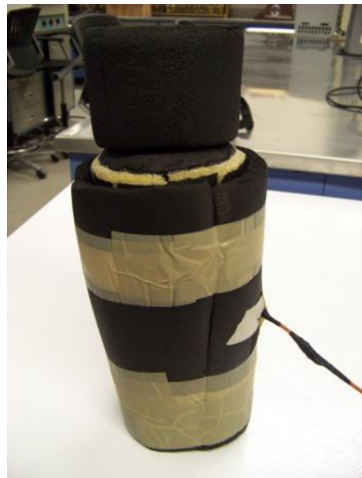
FIG. 3—Martini shaker with insulation and thermocouple wire.
