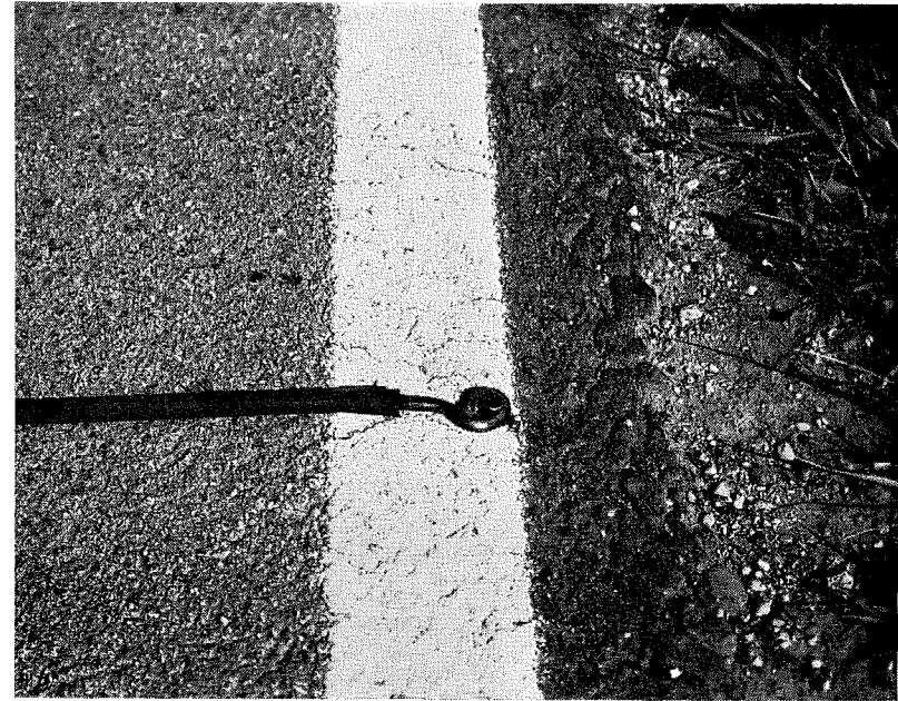
Fig. 15. Detail View Showing Chicago Eyebolt and Roadtube Anchored With Spike Nail at Far-side of Pavement.
