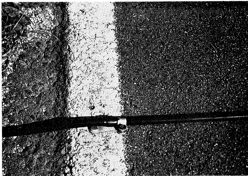
Fig. 17. Detail view of roadtube anchored to near-side of pavement by means of a hose clamp. Small washers are used as spacers to hold the clamp open so the roadtube will slide freely through the clamp. Tape wrapped around the roadtube on the near-side of the clamp holds the roadtube tight.
