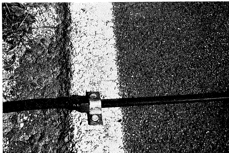
Fig. 18. Detail view of roadtube anchored to near-side of pavement by means of a heavy-duty U-Clamp and a nut slipped over the hose. Tape wrapped around the roadtube on the near-side of the nut holds the roadtube tight.
