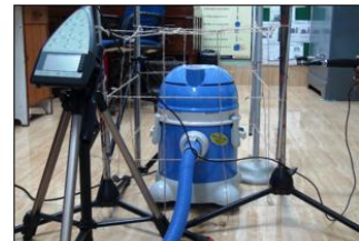
Sound Power Measurement of Vacuum Cleaner
