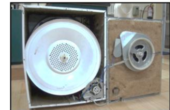
Jute Lined enclosure for noise control of clothes
