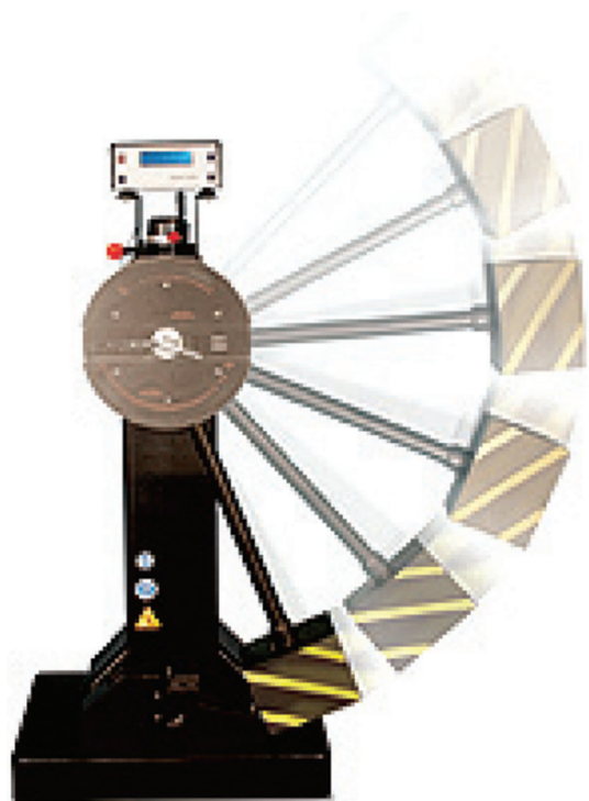
Figure 1.6 Charpy impact test apparatus (courtesy of AWS).
