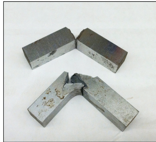
Figure 1.8 Brittle and ductile fracture of CVN specimens.
