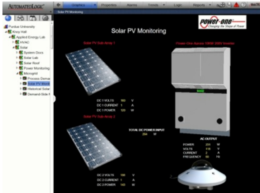
Figure 3.4 WebCTRL Graphic View of Solar PV Monitoring
