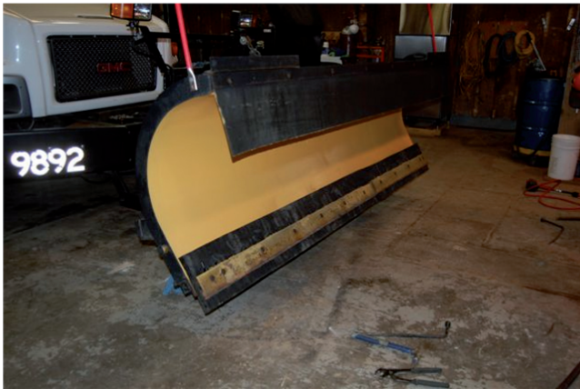
Figure 2.4 Image of full rubber cutting edge (Resolute Rubber, 2013).
