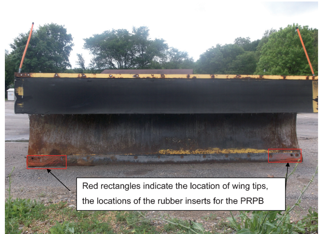
Figure 2.3 Image of INDOT plow showing location of rubber inserts.
