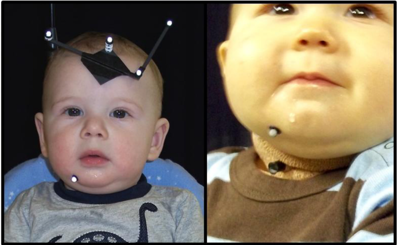
Figure 1. Head block array and jaw marker (left); Jaw marker and laryngeal accelerometer (right)
