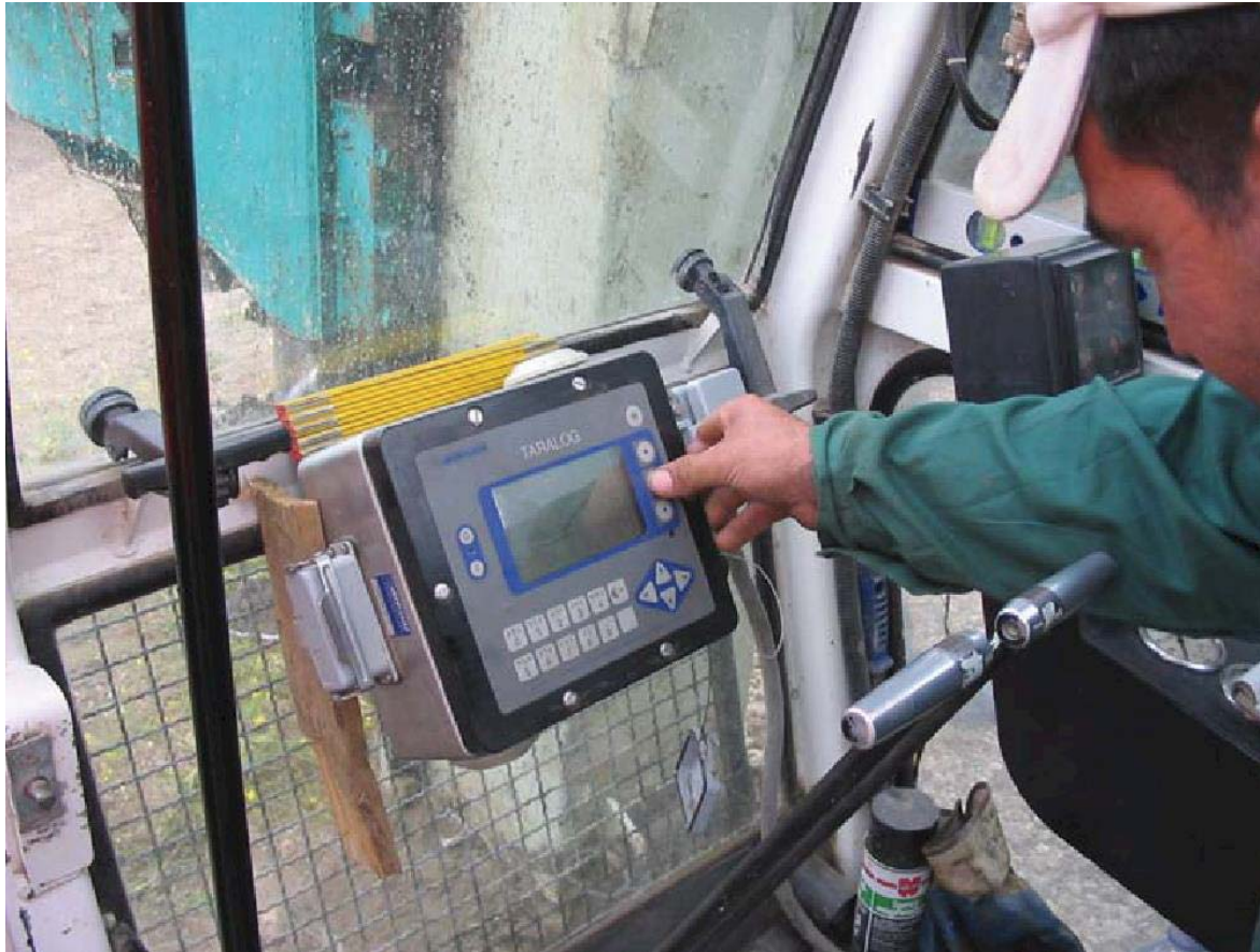
Operator with Cab Mounted Display Used to Control Drilling
