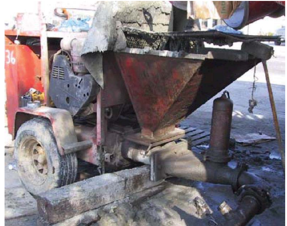
Close up View of Grout Pump
