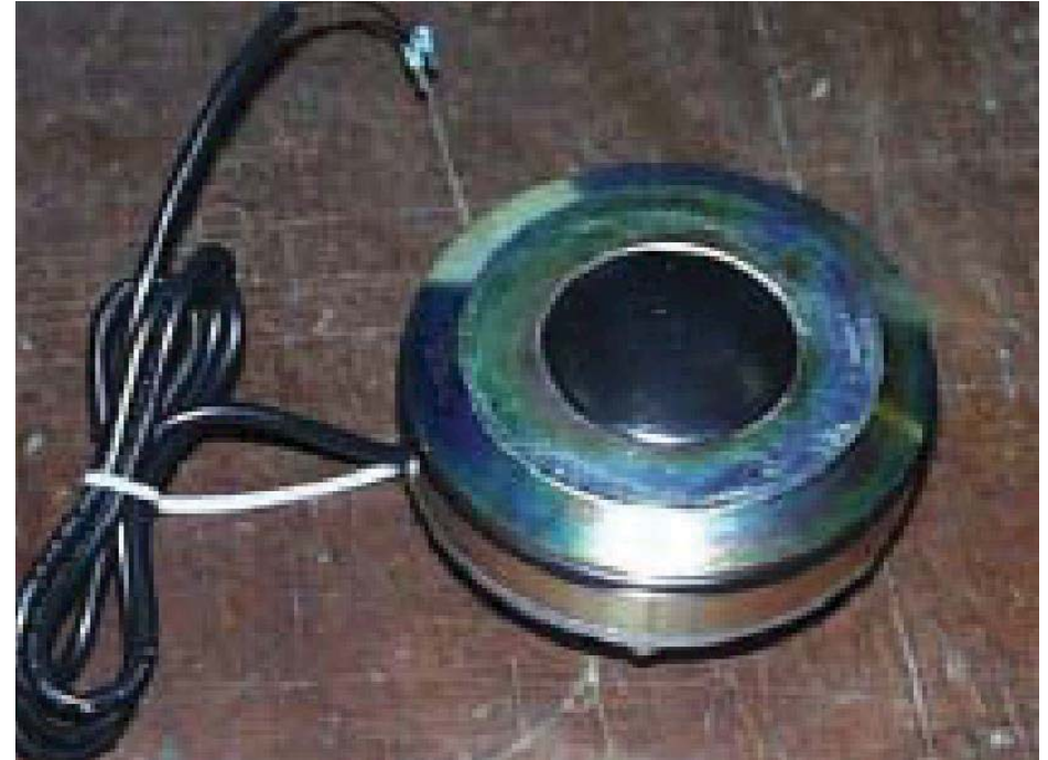
Sensor for Concrete Pressure at Auger Tip
