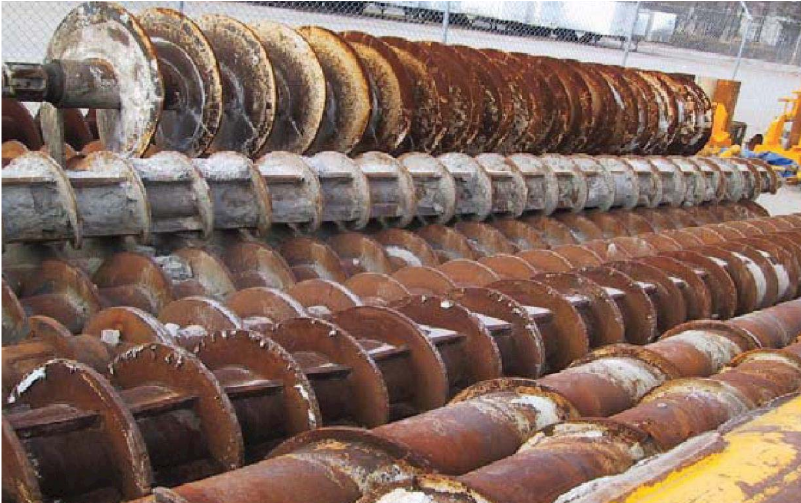
Augers for Different Soil Conditions: Auger for CFA Piles in Sandy Soil (Top) and Augers for DD Piles (Bottom)
