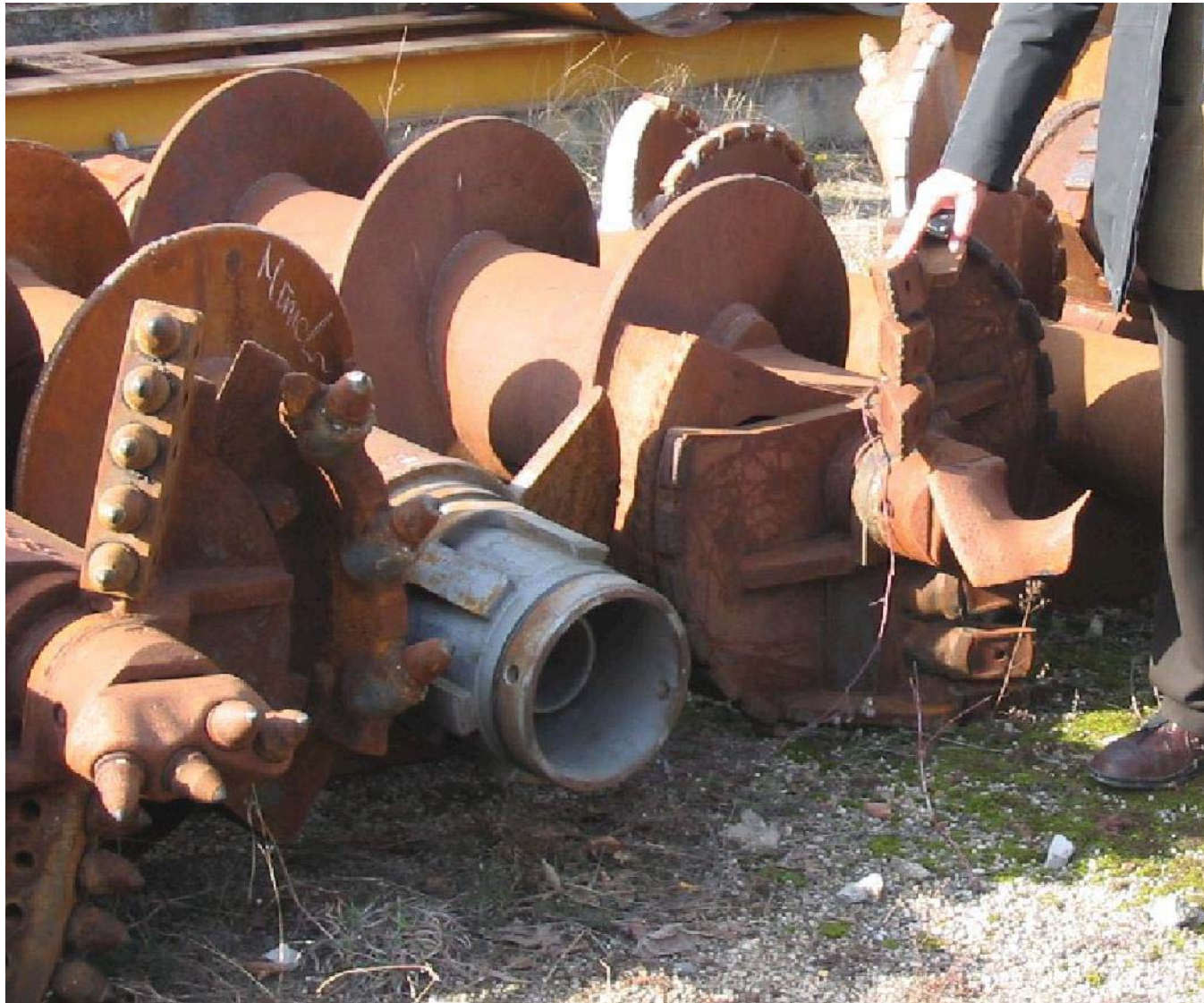
Cutter Heads for Hard Material (left) and Soil (right)
