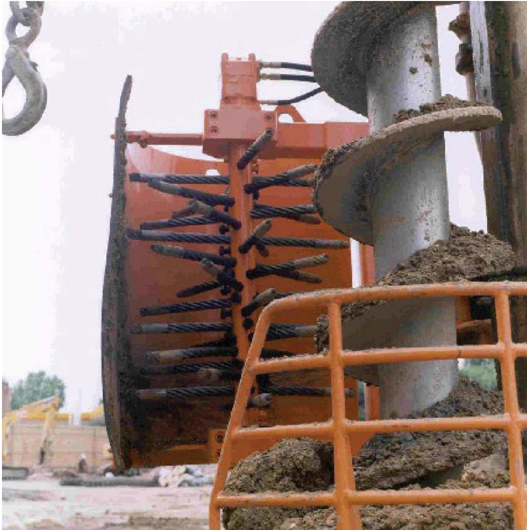
Auger for Use in Clay, with Auger Cleaner Attachment
