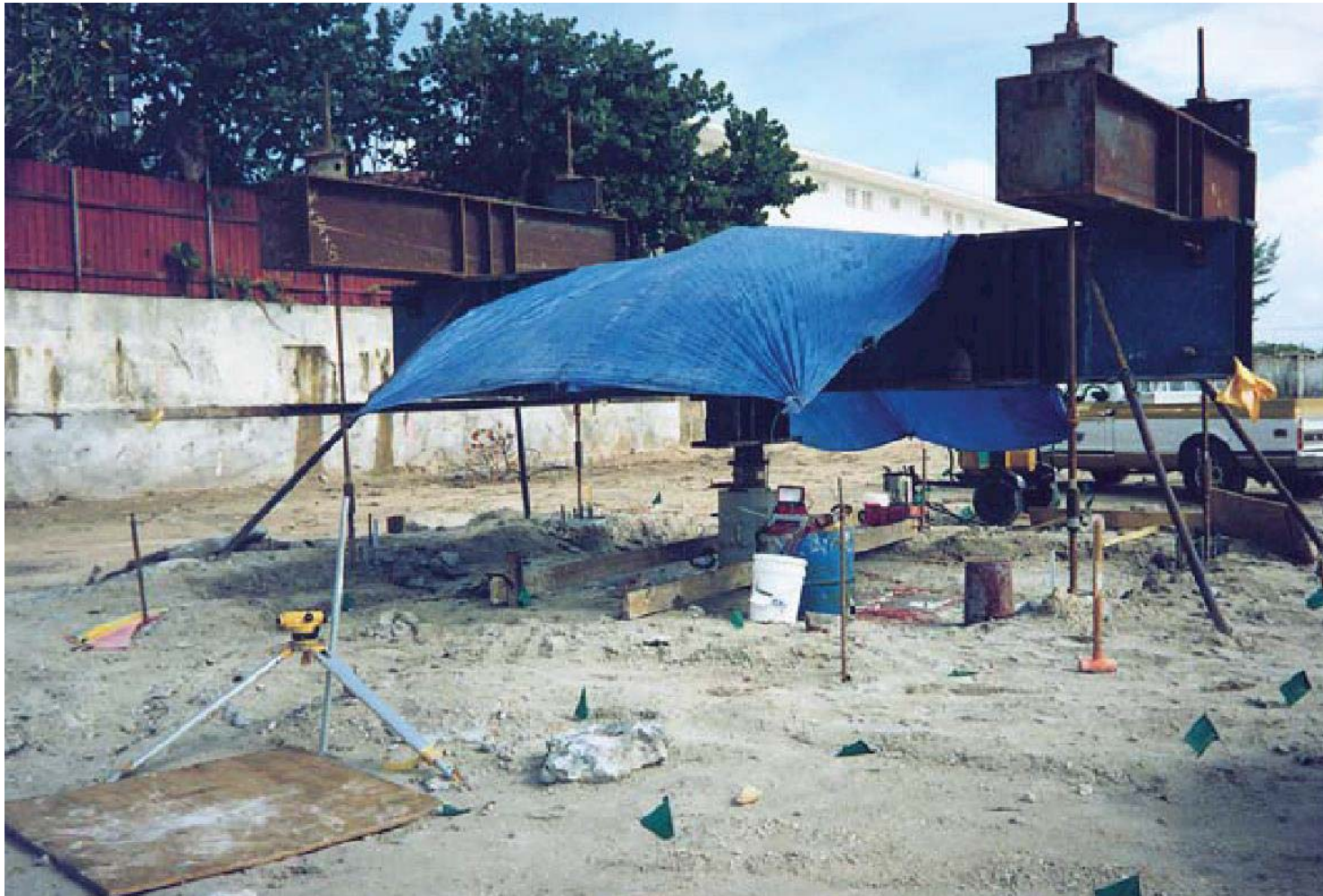
Static Load Test Setup on CFA Piles
