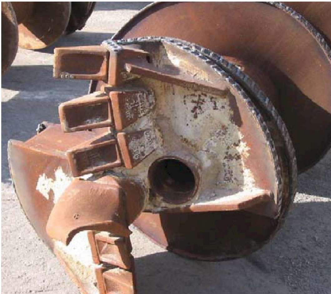
Hole at Base of Auger for Concrete
