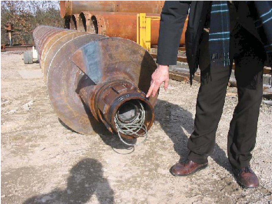
Sensor for Concrete Pressure at Auger Tip
